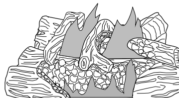
Figure 55 - Typical Flame Pattern for (V)T32 and (V)T36 Series Models
